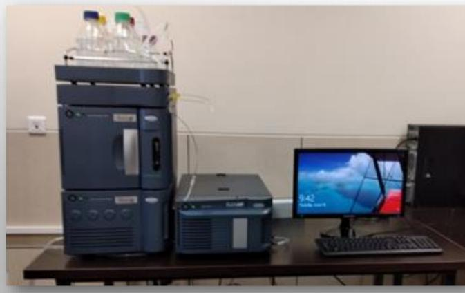
Device Model: ACQUITY UPLC H PLUS / ACQUITY QDa Mass Detector Made by WATERS Company in America
